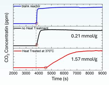
Dynamic CO<sub>2</sub> Breakthrough Curves of blank reactor(blue), 13X zeolite without(black) and with
